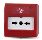
TFB-3168 has been designed to be used with all brands of conventional fire alarm systems and comply with EN54-11. Internal 470-ohm resistance allow ease of installation. It has resettable operation structure which can be reset by using a special plastic key.
