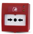
TWB-1966 is a wireless manual call point used to create manual warning in case of fire. It supports resettable type of operation and additional protection cover can be implemented to avoid situations that may cause false alarms.
